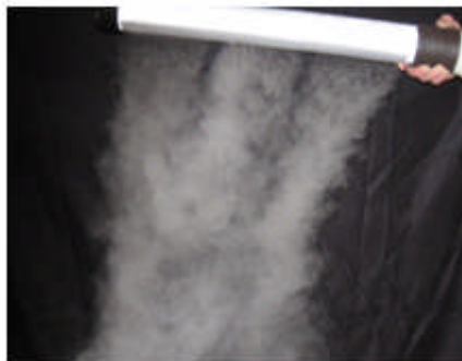
Optional Fog Curtain Wand to reduce pressure out & create wide Fog Curtain to Visualize Airflow
